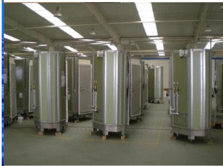
TNF Wet Units are made with a special focus on details to ensure that form, function and durability contribute to the overall effect. The TNF Wet Units are made as pre-fabricated ready-to-install modules or as knock-down kits. In our design we focus on long lasting solutions which will give the user maximum comfort. The wall surface is coming in TNF Magic, PVC, stainless, painted or tiles.
